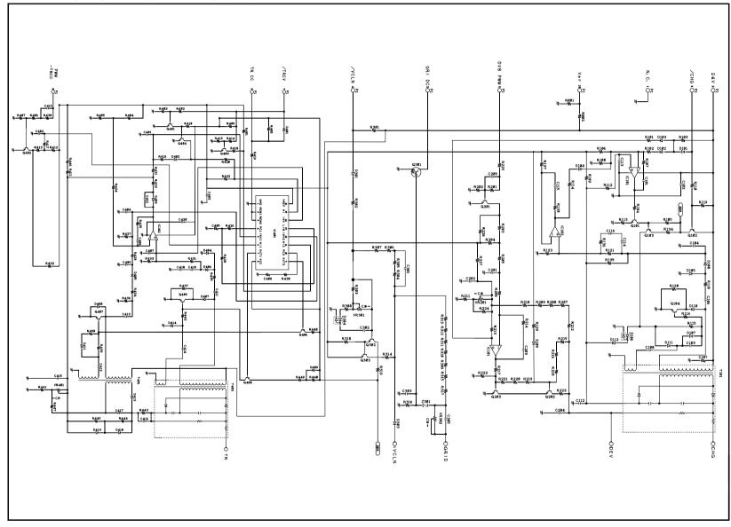
Appendix 4.19 High-voltage Power Supply PCB Circuit Diagram (100V)
