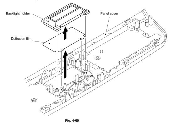
(5) Remove the backlight holder and the deffusion film.
