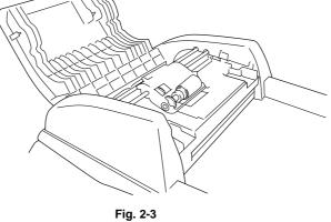
(2) Slide ADF support into the groove on ADF.
