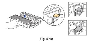
(7) Clean the primary corona wire inside the drum unit by gently sliding the blue tab from right to left several times. Return the tab to the home position before you put the drum unit back in the machine. If you do not, printed pages may have a vertical stripe.
