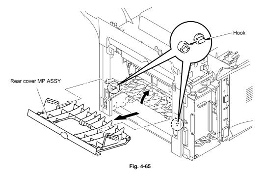
(2) Remove the outer chute MP ASSY.
