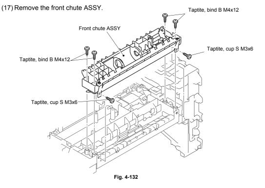
(16) Remove the two cup S M3x6 Taptite screws and the four bind B M4x12 Taptite screws.
