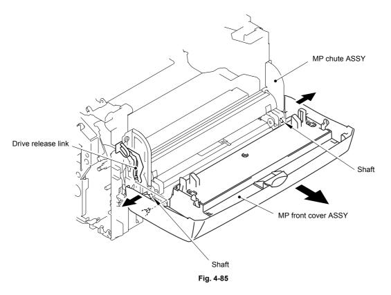
(8) Remove the shaft of the MP front cover ASSY from the drive release link, and then remove the MP front cover ASSY from the MP chute ASSY.
