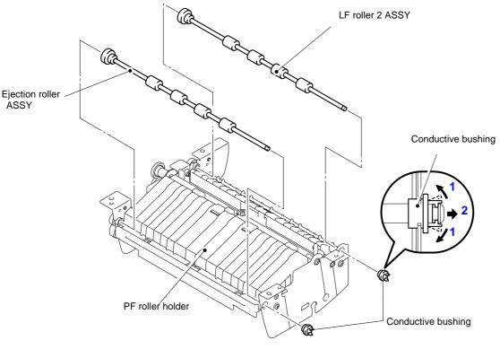
(28) Remove the conductive bushing, and then remove the LF roller 2 ASSY.
