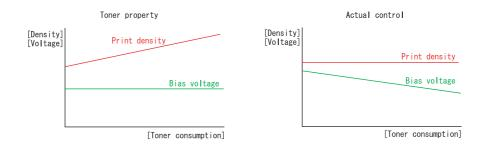
To correct this problem and maintain the steady print density, the machine counts the printed pages after the toner cartridge is replaced and changes the bias voltage according to the number of the printed pages.
