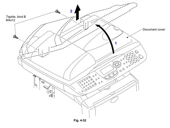
(4) Remove the two bind B M4x12 Taptite screws, and then remove the document cover.
