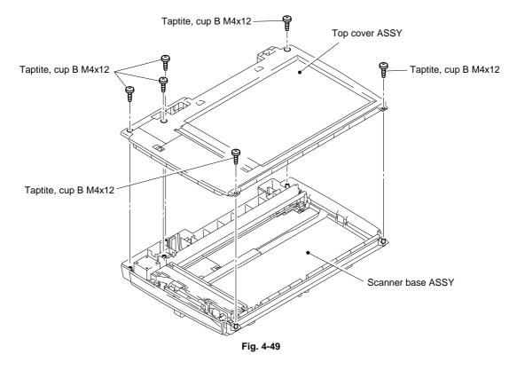
(5) Remove the six cup B M4x12 Taptite screws, and then remove the top cover ASSY.
