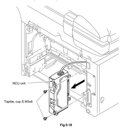
8) Remove the two cup S M3x6 Taptite screws, and then remove the NCU unit.
