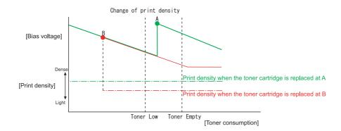
In order to deal with this unexpected usage and maintain the steady print density, the machine can be initialized the developing bias compulsorily in the following procedure.
