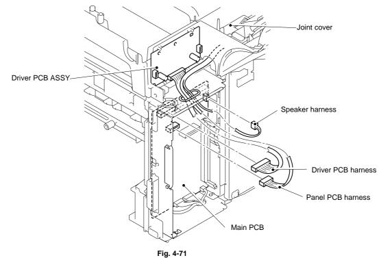
(2) Remove the four bind B M4x12 Taptite screws, and then remove the joint cover.
