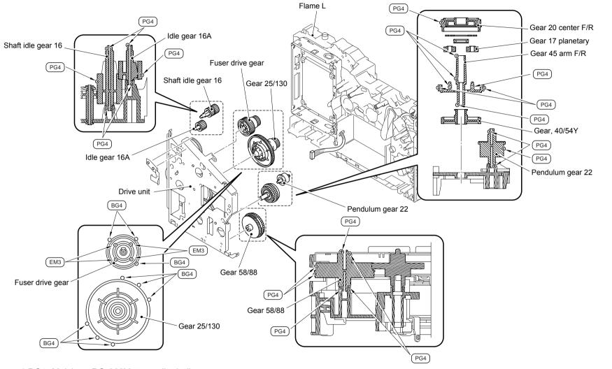
\* PG4: Molykote PG-662Y 4 mm dia. ball BG4: Grease BG999 4 mm dia. ball EM3: Molykote EM-D110 3 mm dia. ball
